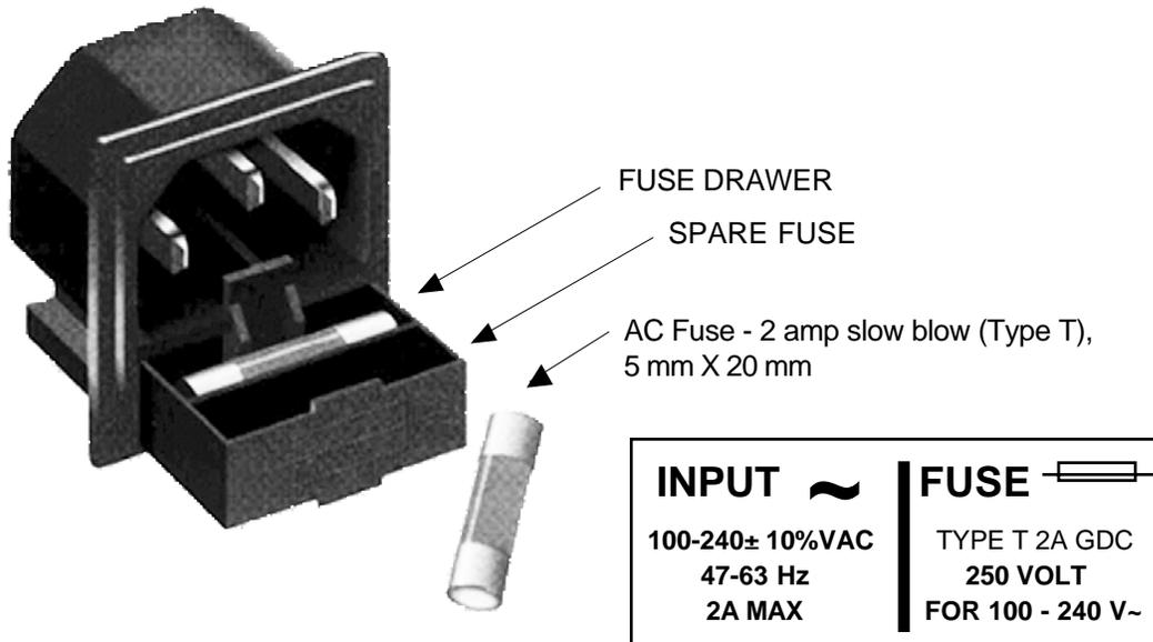
**FIGURE 2.5 Fuse Location and Spare Fuse**
